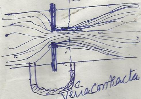
It is a variable head flow meter. It meets the objections to the venturi but at the price of a larger power consumption.
