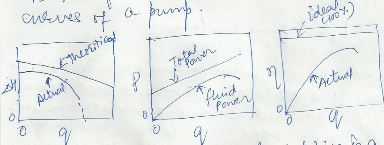
The theoretical head-flow rate relation is a straight line, the actual developed head is considerably less and drops to zero as the rate increases to a certain value in a given pump.
